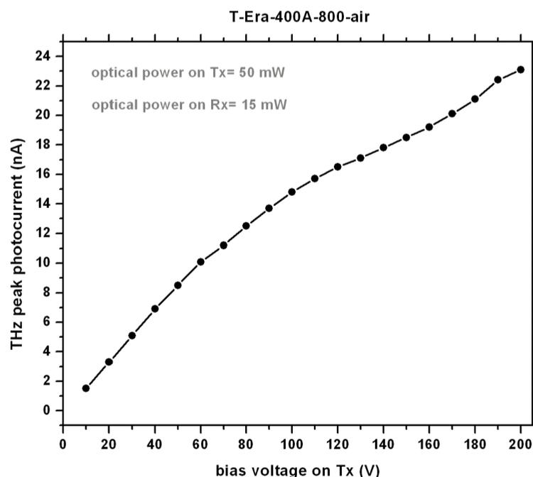
Figure 6. Terahertz peak photocurrent on T-Era-20D40P-800-air receiver versus bias voltage over the transmitter T-Era-400A-800-air.
