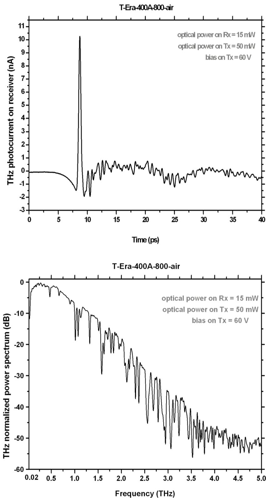
Figure 4. Typical THz pulse and its corresponding normalized power spectrum generated by a T-Era-400A-800-air transmitter module and detected by a T-Era-20D40P-800-air receiver module.
