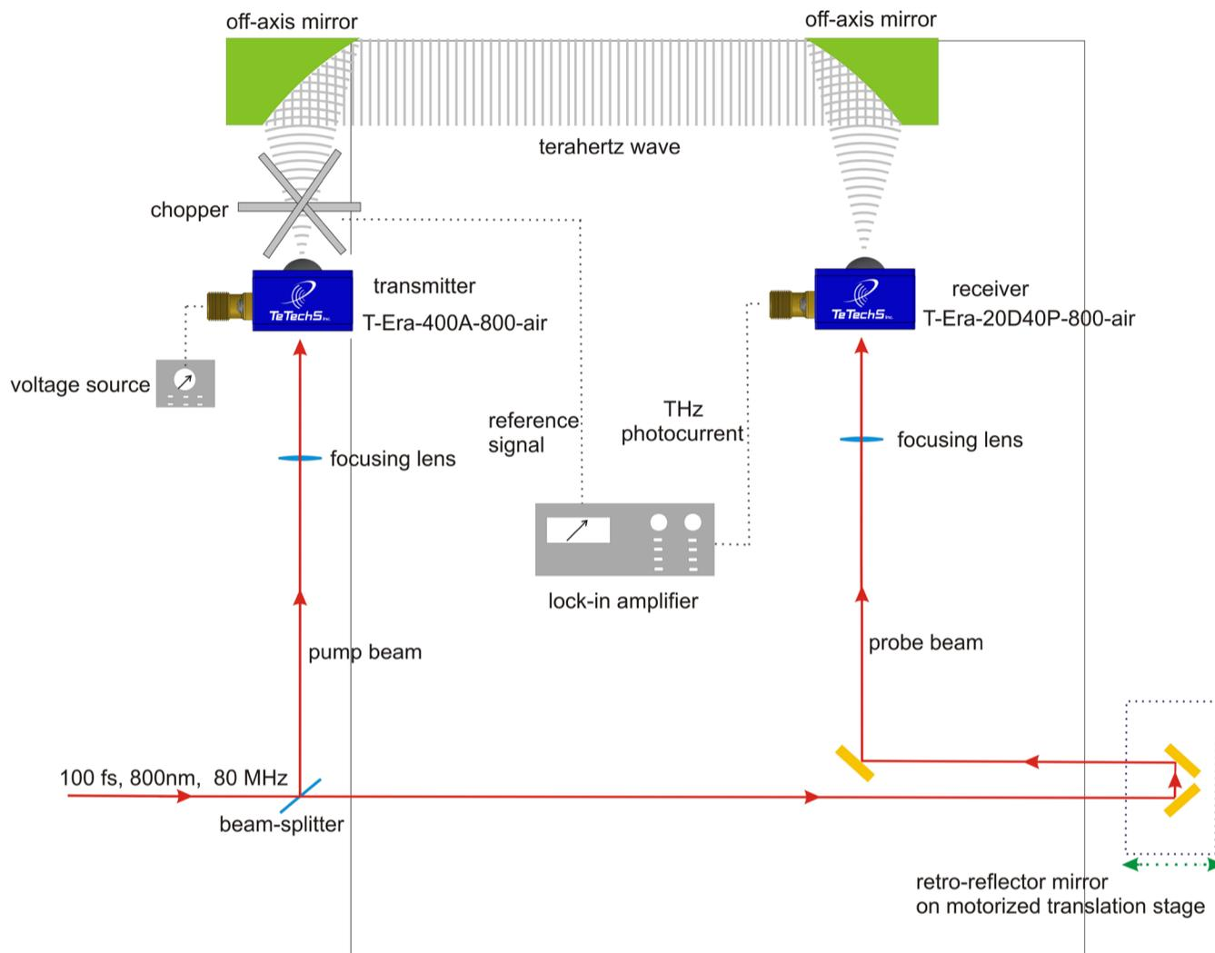
Figure 3. A terahertz response measurement setup for T-Era-400A-800-air THz-PCA.
