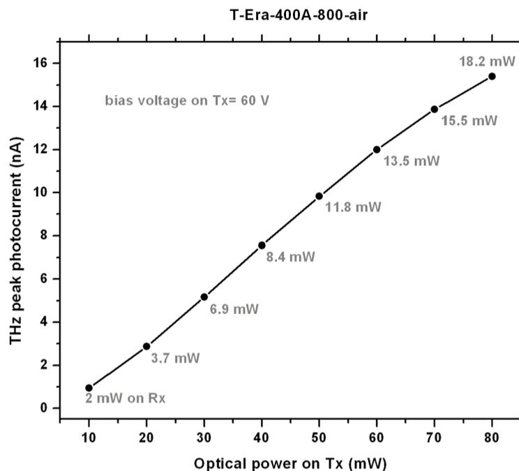
Figure 5. Terahertz peak photocurrent versus average optical power over the T-Era-400A-800-air THz-PCA. The average optical power on the receiver module for each measurement point is shown on the graph.
