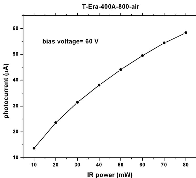
Figure 2. Photocurrent versus average optical power over the T-Era-400A-800-air THz-PCA.
