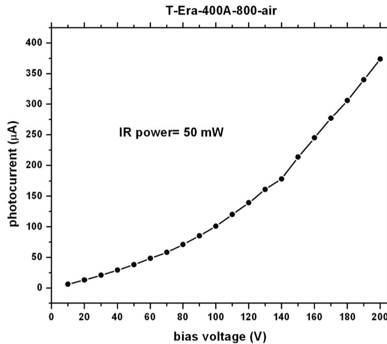
Figure 1. Photocurrent versus applied bias voltage across the T-Era-400A-800-air THz-PCA.
