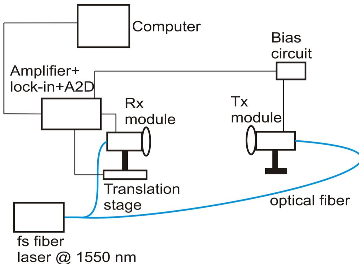
Figure 2. A terahertz response measurement setup for T-Era-100A-1550-fiber THz-PCA.
