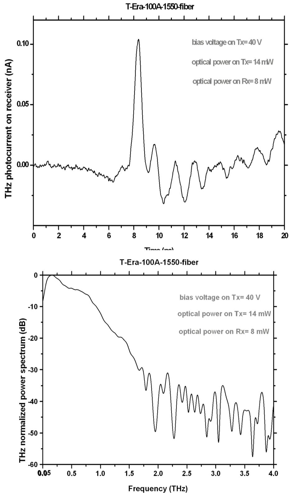
Figure 3. Typical THz pulse and its corresponding power spectrum generated by a T-Era-100A-1550-fiber transmitter module and detected by a T-Era-20D40P-1550-fiber receiver module.
