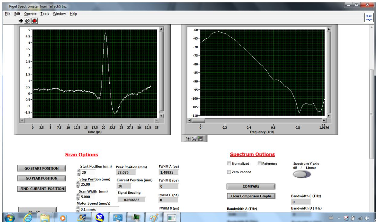
It is shown that the pulse is broader from 1.3 ps in freespace to 1.5 ps with the ABS sample and the peak position shifted to 23.08 mm. There is also attenuation due to the sample.
